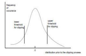
Fig. 1. The clipping method after initial retinex operation illustrated on histogram.
